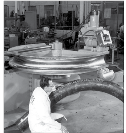
Pines Model 8 with Integral Damp Die for Large Radii
