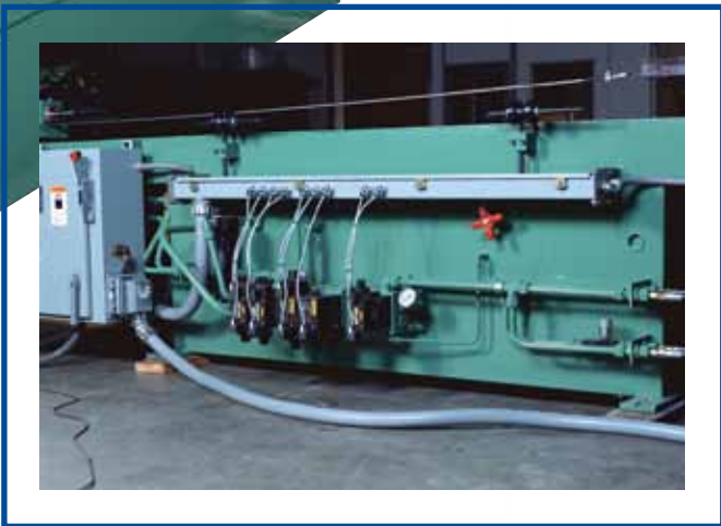
Outside hydraulics provide ease of maintenance.
